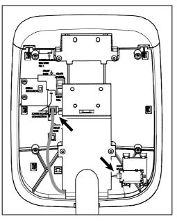
Figure 17: Routing the data and heart rate cables
